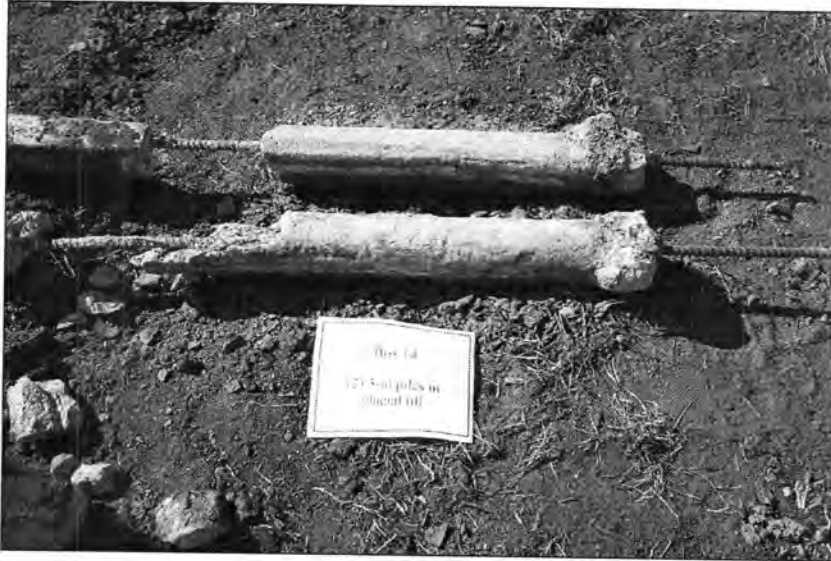
Figure 177 – (2) Exhumed 127-mm Piles (Pile 14 A and 14 B)
