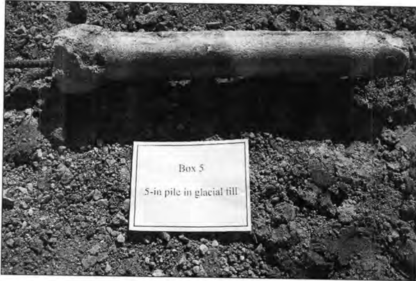
Figure 175 – Exhumed 127-mm Pile (Pile 5)
