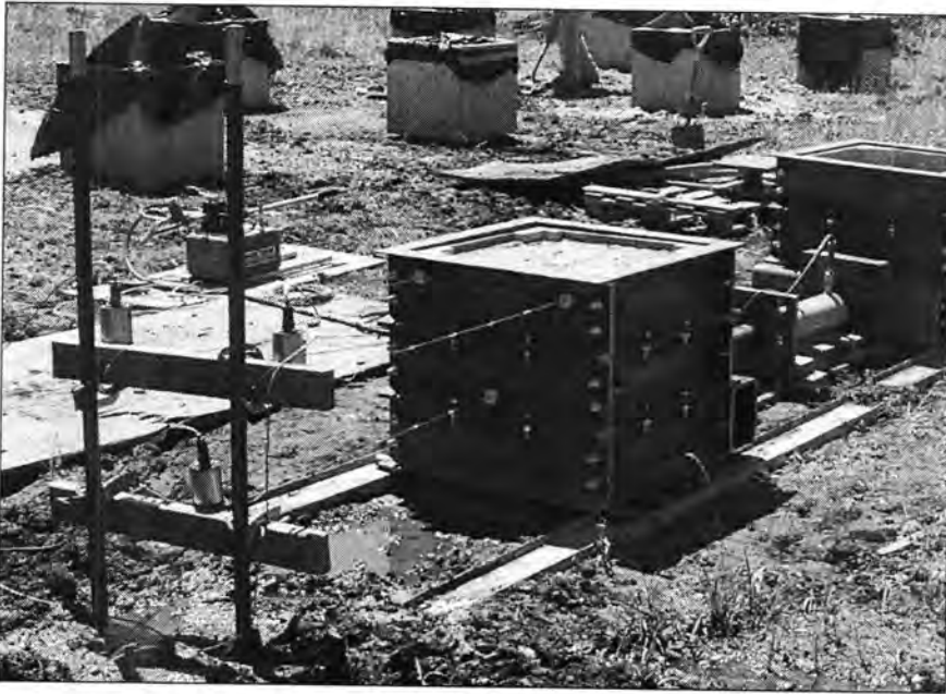
Figure 53 – Displacement Gauge Locations on Shear Boxes
