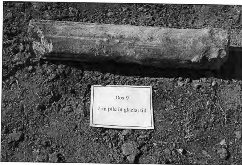
Figure 176 – Exhumed 178-mm Pile (Pile 9)
